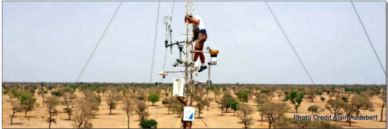
Fig. 1a: Eddy covariance tower and meteorological instruments over an agro-sylvo-pastoral parkland dominated by Faidherbia albida . Photo by Alain Audebert, end of the dry season.
