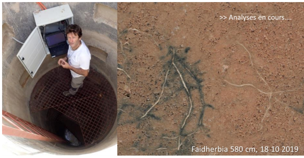
Fig. 3. Root mini-rhizotrons tubes set up in 2019 in Sob ( Faidherbia Flux ) site in Senegal
